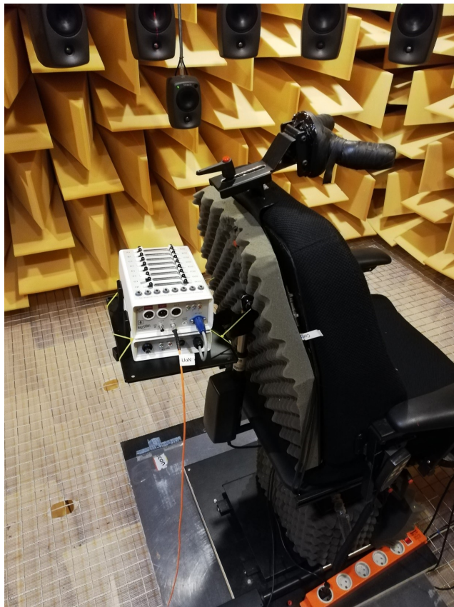
Figure 4.5: Setup inside anechoic room (Motorized chair, adjustable neck support and EEG equipment).
